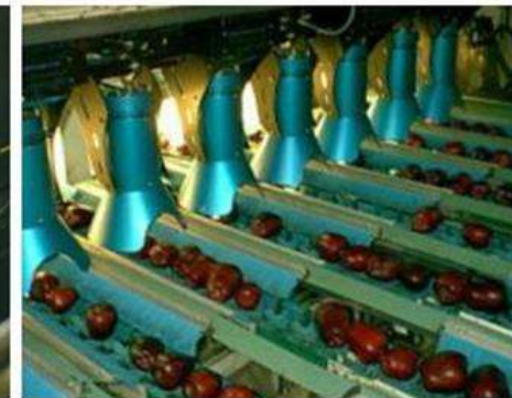
Modern grading machine based on weight and Brix (TSS)
