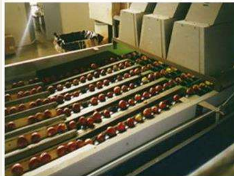
Modern grading machine based on weight and Brix (TSS)
